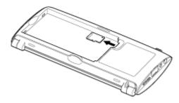
6. Hold the microSD memory card by the both sides, and pull it out of the slot.
